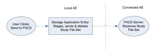
VMS operator initiates a "Send to PACS" command for a specific study in the study list in VMS GUI application. As a result, VMS Local AE stages, sends the corresponding study to the configured PACS server; and finally cleans up the staged file-set files.
